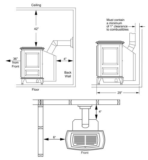
Figure 3 - Clearances for Standard Installation
